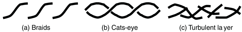
FIG. 3. Classification of the structures observed frequently within vertical shear RHIs. The lines show the patterns of maximum shear. Braids, cat’s-eyes and a turbulent layer are represented in (a)–(c), respectively.
