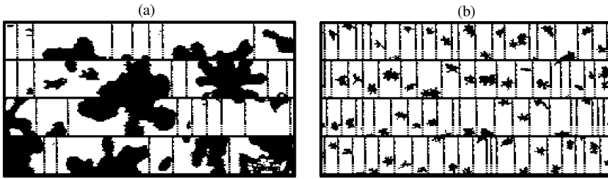
Figure 6. Crystal images from the two-dimensional (2D) cloud probe (a) and 2D precipitation probe (b) beneath the high- Z_{DR} region that was shown in Fig. 5(f), 15 km from Chilbolton at an altitude of 4 km. The array width of the 2D cloud probe is 800 \mu\text{m} and that of the 2D precipitation probe is 6400 \mu\text{m} .
